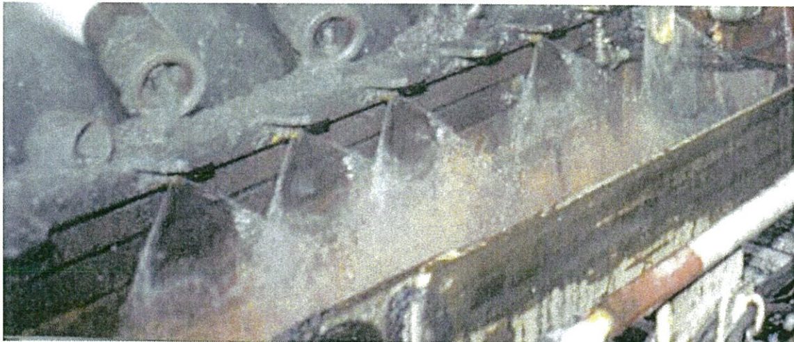
Headgate splitter arm with flat-fan sprays mounted on gob side of belting.
