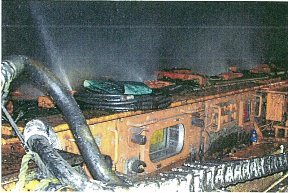
Directional sprays mounted on face side of shearer body
