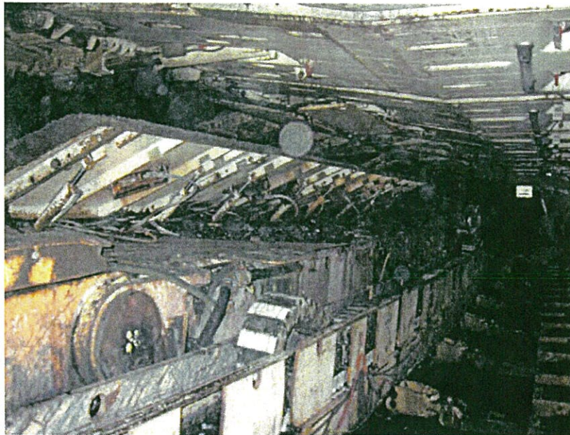
Raised deflector plate can enhance the effectiveness of the directional spray system.
