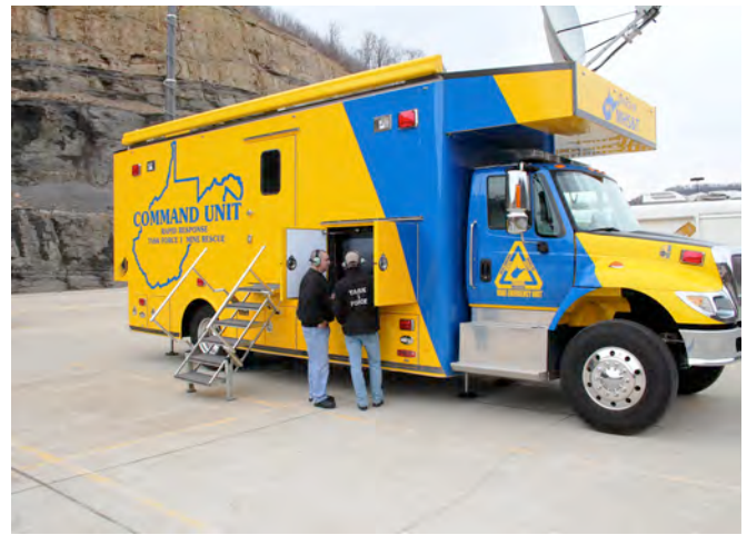
SatCom 1 mobile command unit supports mine rescue training in gas analysis & weather detection (lightning). It includes radio & video communications to support fully function MERD exercises.
