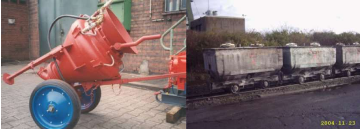
Figure 12: Small (left) and Large (right) Compressed Air Duster Units. Source: RAG Hauptstelle für das Grubenrettungswesen (RAG Mine Rescue Headquarters), Herne, Germany
