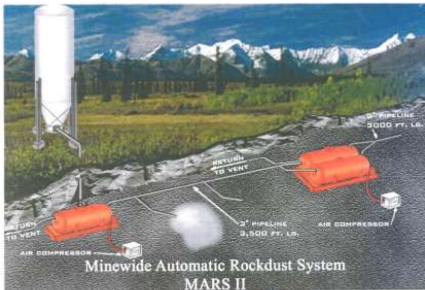
Figure 11: Mine-wide automatic rock dust system, (A.L. Lee corporation, www.alleecorp.com )
