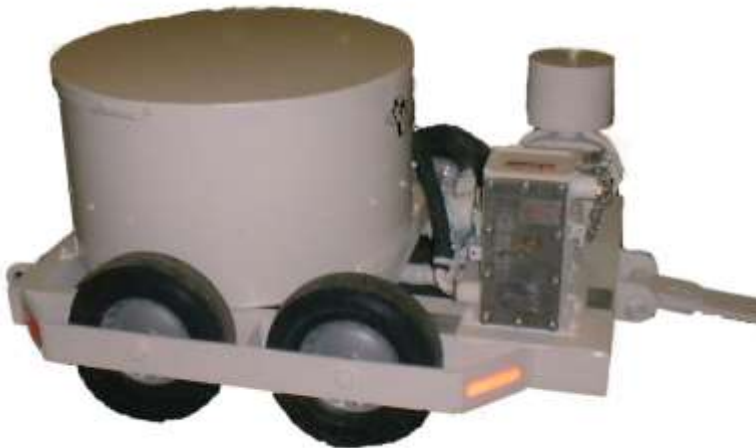
Figure 13: Rubber-tire mounted trickle duster commonly found in US mines (A.L. Lee Corp.; www.alleecorp.com ).
