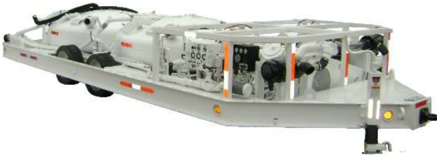
Figure 10: Wheel mounted bulk rock duster (A.L. Lee Corp.; www.alleecorp.com )
