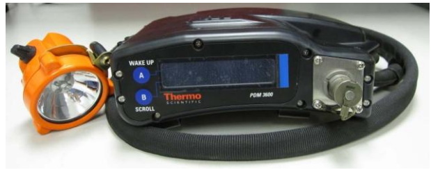
A continuous personal dust monitor. The monitor is worn on your belt, and an intake valve next to the lamp collects the dust to be measured.
