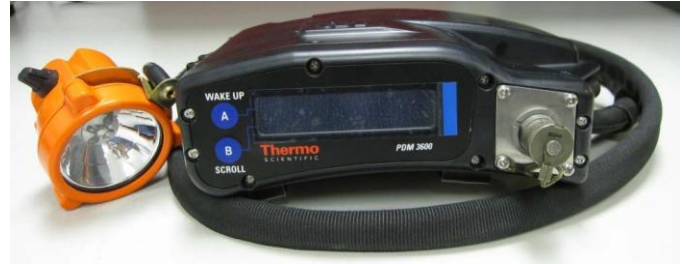
The Thermo Fisher Scientific PDM 3600 continuous personal dust monitor.
