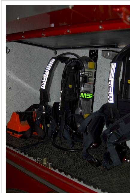
SCBA packs carried on a rack in a firetruck
