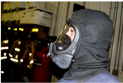
A person wearing an MSA Brand breathing mask with a Nomex hood on. This face piece attaches with a regulator to form a full SCBA.
