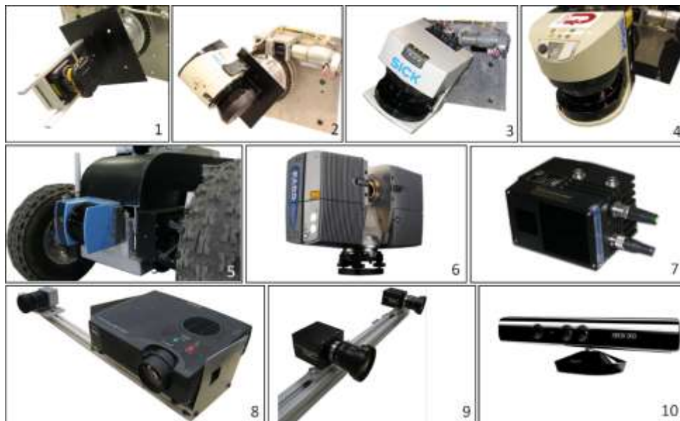
Figure 5. Illustration of Evaluated Sensors and Configurations – (1) rotating Hokuyo UTM-30LX, (2) rotating SICK LMS111-10100, (3) rotating SICK LMS291-S14, (4) rotating SICK LMS511-10100, (5) rotating SICK LMS200-30106 affixed on a mobile robot, (6) Faro Photon80, (7) IFM O3D 201, (8) custom structured light sensor, (9) custom stereo vision sensor and (10) Microsoft Kinect.
