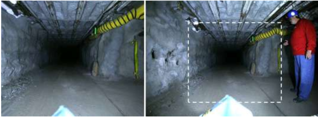
Figure 28. Images from a standard 90 degree "wide angle" lens (left) versus a 180 degree fish eye lens (right) illustrate the enhanced situational awareness in fish eye optics.
