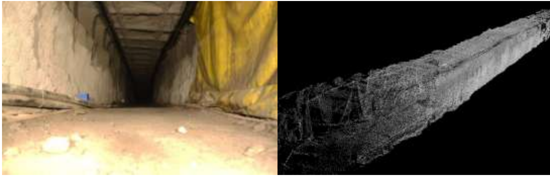
Figure 15. Unstructured Corridor photograph (left) and point cloud (right). Blue calibration cubes are visible in the image.
