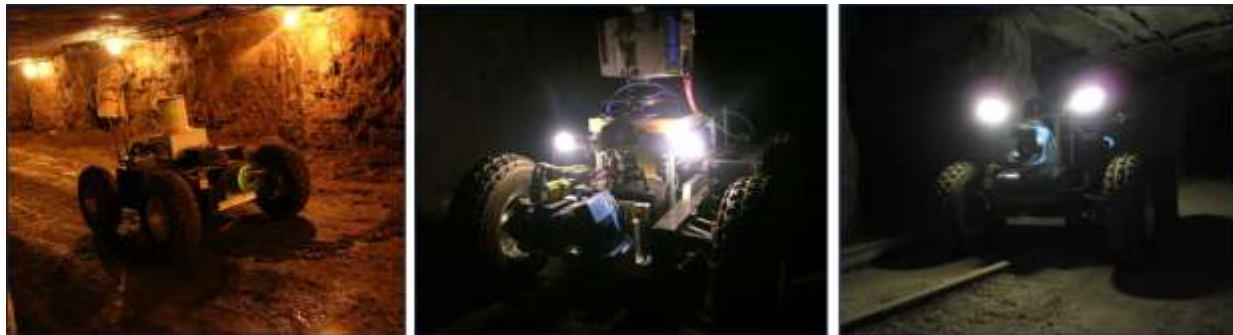
Figure 23. The Robot scout platform is configurable with a spectrum of sensors suited to each task: 1) radar configuration for smoke-filled response, 2) mounted with survey scanner for inspection modeling and 3) reconnaissance scout.
