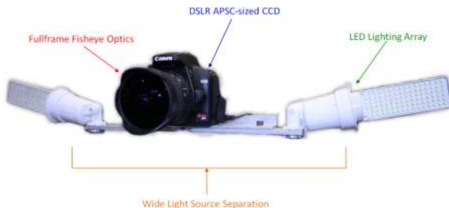
Figure 27. Configuration of Imaging Sensors on Robot scout
