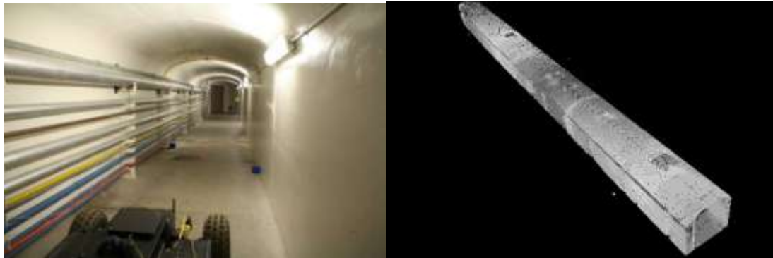
Figure 16. Structured Corridor photograph (left) and point cloud (right).
